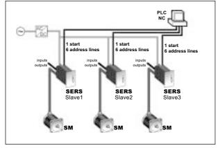
Operation with a PLC/NC or simple switches as higher order control, which call and start different operational programs in the SERS via the digital-parallel inputs (binary mode). Up to 64 different operational programs per SERS can be called.
