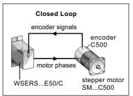
By using Closed Loop control the stepper motor can be operated always with its maximum torque.
