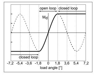
As long as the load angle is  $<1,8^{\circ}$ , the stepper motor will be operated in open loop mode. If the load angle is  $\ge 1,8^{\circ}$  (in open loop the motor now would loose its position) the stepper motor will be operated automatically in »closed loop mode«.
