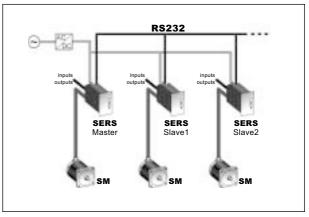
Operation with a SERS as higher order intelligent control (master), which controls other SERS-slaves via the serial interface.
