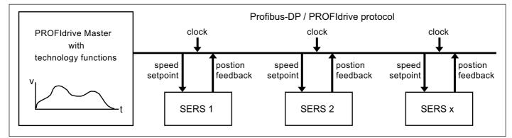
A motion profile for multiple axis (e.g. an interpolation in a 3D system with X-Y-Z axis) is given to a PROFIdrive master.
